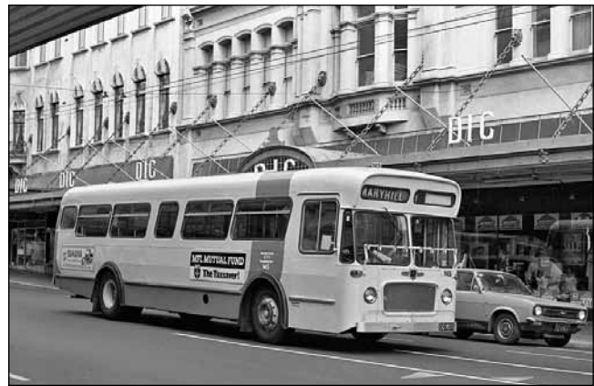
Leyland Panther PSUR1B/2R No.145 The front mounted rail was for the carriage of prams and pushchairs. Note the earlier type of wheel nut guards Sean Millar)
