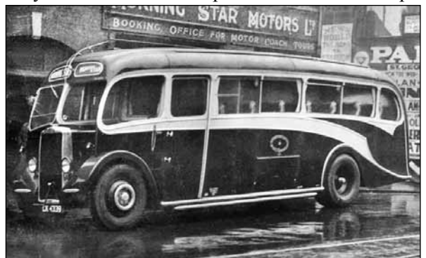
CK 4339 with Morning Star with its new body. Note the hinged panel at the front nearside to mimic a full-front; it probably rattled in service and would have been a nuisance when carrying out maintenance (Mike Sutcliffe collection)
