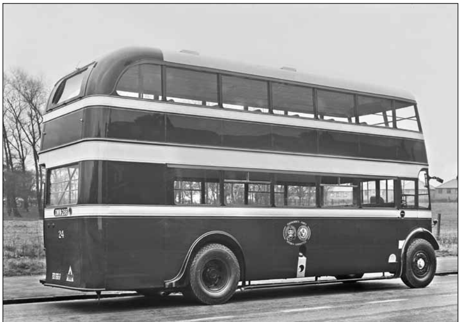
A rear view of No.24, DWV 266, with its moulded rubber rear mudguards and swept-out rear lower panel, on which was the Dewandre transfer, a triangle warning about the ferocity of vacuum powered brakes. The three cream bands were profusely lined out in green and the roof was Ivory-coloured (possibly white lead paint)
