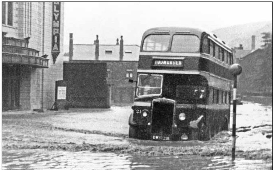
Leyland Titan TD7, No.21, DWY 391, with Massey body carefully passes the Olympia Cinema in the regularly occurring floods along the Burnley road when the River Calder burst its banks (Mike Sutcliffe collection)
