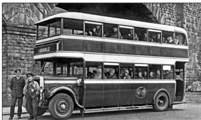
WX 2074 , one of the two supernumerary TD1s which were brought back into the main fleet thereby extending their lives to 18 years, rather than the standard 10-year life normally aimed for by TJOC. Driver Alva Brown, Conductor Harry Escritt (Mike Sutcliffe collection)
