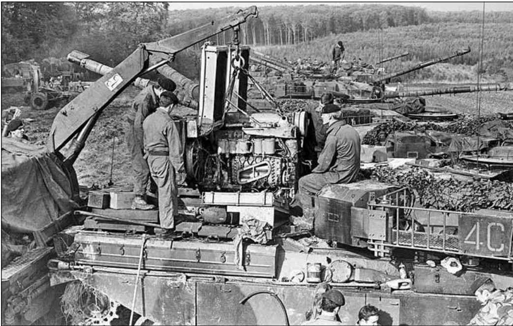
A powerpack change underway, the two radiators are in the upright position to assist with removal. The lobes inside the scavenge blower can clearly be seen, in the vehicle these would be covered by the air cleaner. The powerpack is being lifted by an FV434 Armoured Recovery Vehicle, this was capable of lifting the Centurion and Chieftain engines but not the Perkins engine fitted to the Challenger. This image is from the Richard Rose collection provided courtesy of the 14th/20th King's Hussars Regiment Club website
