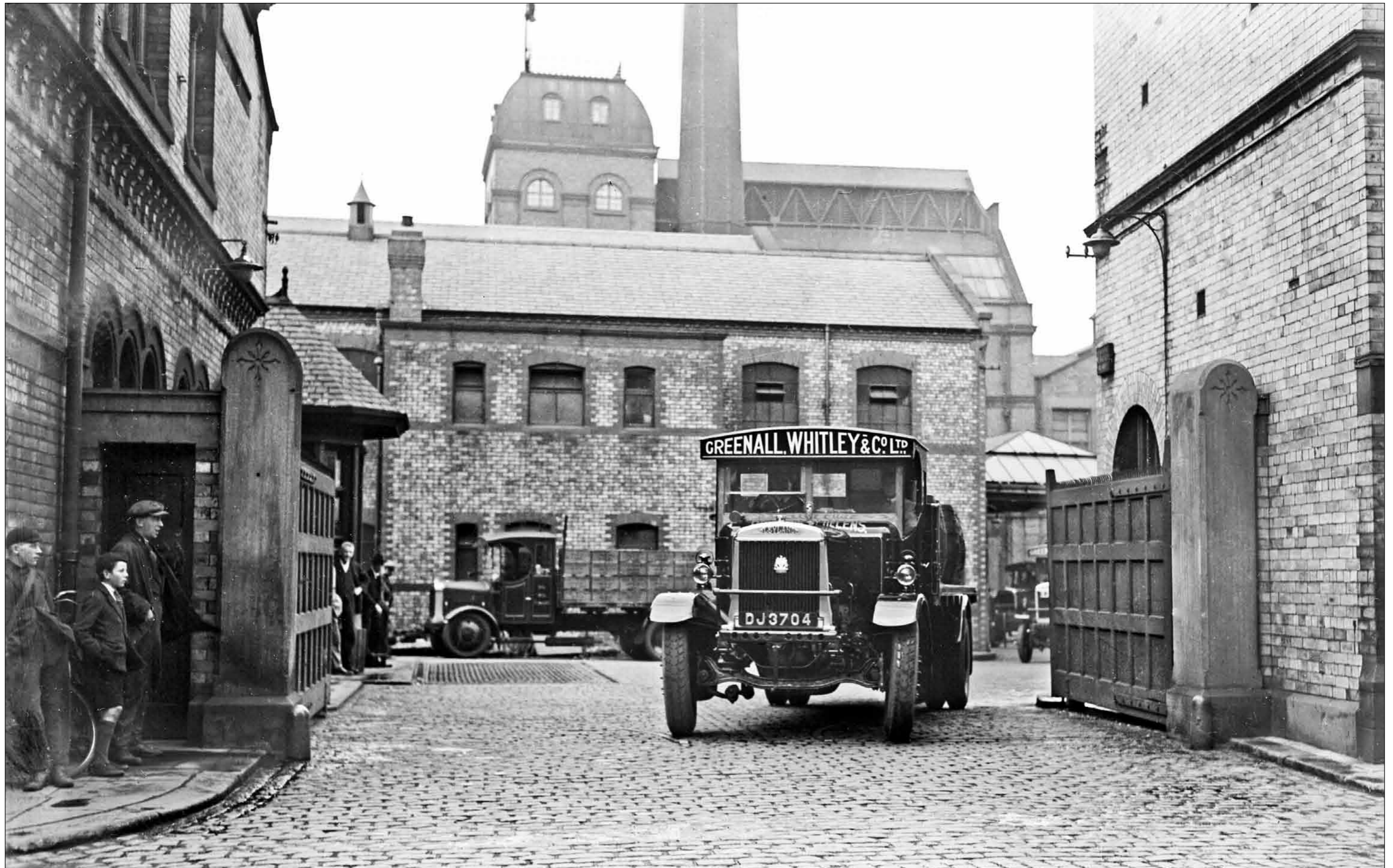
Greenall Whitley of St Helens were loyal Leyland customers, going back to the days of their Leyland steam wagons. This Leyland GH6 (4-tonner) was one of two, chassis nos.13919/20, bought in July 1928 and on 4 x 8 pneumatics (24in wheel centres). It is easily recognisable as a late GH, with the Ricardo headed E.36/2 engine, due to the blanked-off centre hole on the front crossmember, also the wide front axle beam with extra wide spring saddles (with 2½in flat outside the springs) to enable the same axle to be fitted to the wider framed SQ2. The 5 and 6-ton models PH and QH would look similar, but would have the deeper radiator going below the top of the frame. Their little Z Type is parked behind, possibly needing repairs, a troublesome model! (BCVMT L005183F)
