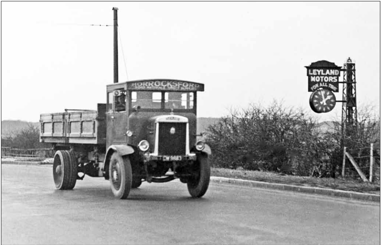
A Leyland SQ2 6/7 Ton lorry, CW 9883, passes the Lea Clock on the Blackpool road in March 1931. Note the pneumatics (40 x 8s) on the front and solids at the rear
