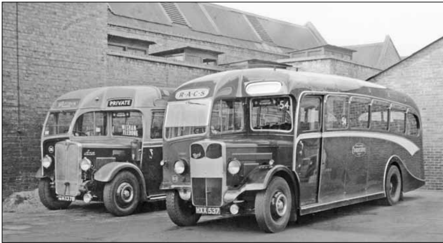
One of the Royal Arsenal Co-op Society AEC Regals with its Beadle body when quite new (AD Packer)
