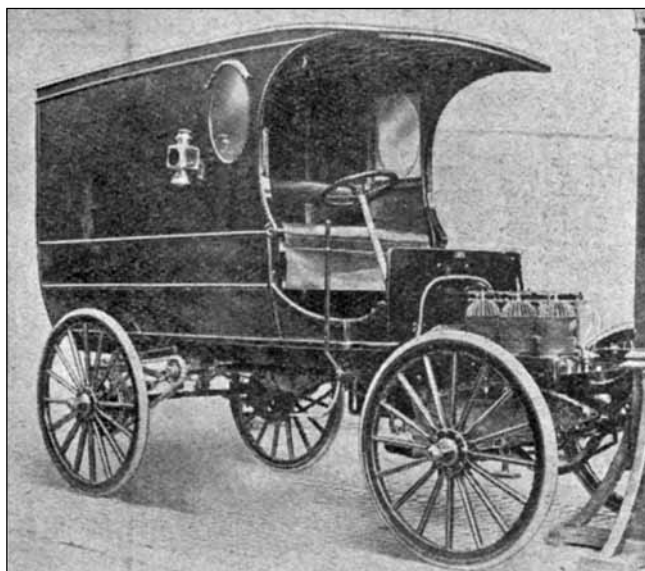
At the Show, the Chase van with bonnet removed showing the air-cooled cylinders (Mike Sutcliffe collection)
