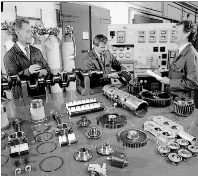
Left – Oman L60 components laid out for inspection in the Test Operations building at Spurrier Works. This posed photo was taken in 1993 shortly after formation of the new company and was used in the marketing brochure. The three engineers in the photo are left to right Terry Higgins (sadly deceased), Mick Boardman and Terry Blackhurst. The large piece of equipment in the background was “my friend” for many years. Its technical name was Gaseous Invisible Emissions Cart used to measure pollutants in exhaust gas, not something they ever bothered about on the L60!
