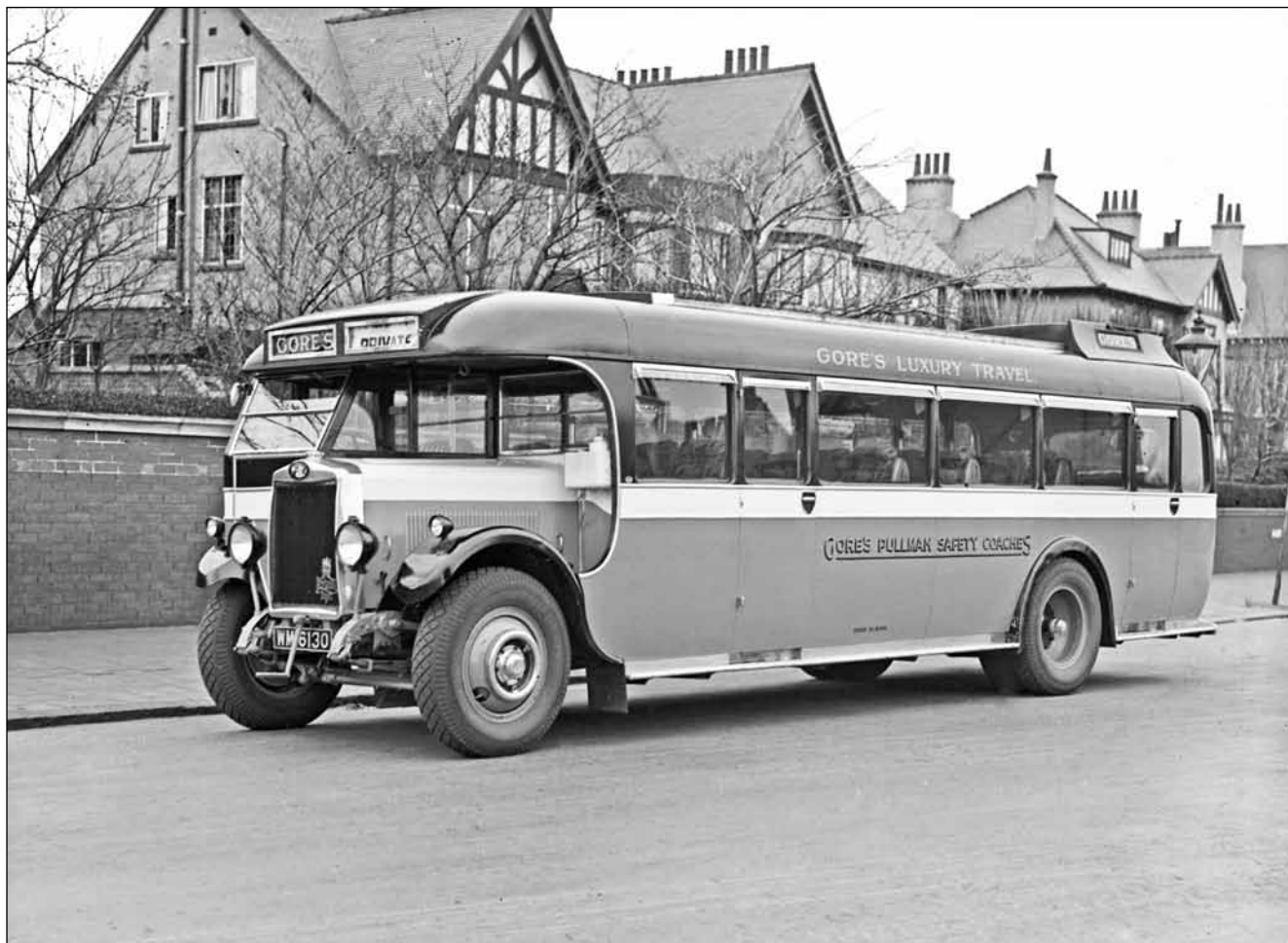
The first Tiger operated by Gore's was this attractive TS1, chassis 61472, with Spicer 30 seat body, new in April 1931 (BCVMT L009246)
