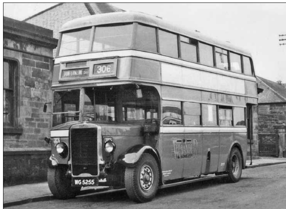
R147 outside Market Street Garage in Dunfermline has a half-and-half body overhaul. The top deck has sliding vents and windows set in Simplastic pans whilst the lower deck retains half drops and original glazing. This work was carried out at the Fife area body shop based at the old Kirkcaldy Corporation Tram Depot at Gallatown.
