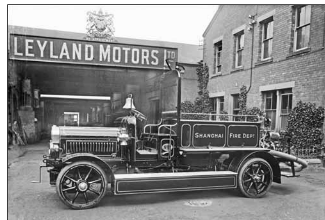
Shanghai's first Leyland, a U.55.V with a 55hp, 10 litre petrol engine, delivered in 1913. It had been exhibited at the 1913 Commercial Motor Show (BCVMT LB1310)
