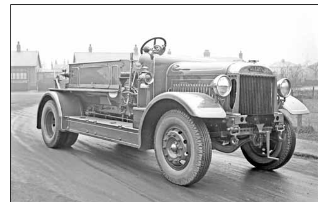
Shanghai's final Leyland was the ex-Lever Brothers FE.U4 seen here in 1933, having been modified by Leyland Motors and on pneumatics (BCVMT L013700)
