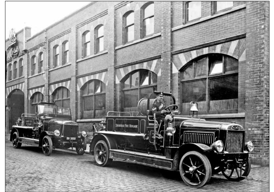
In April 1921, Shanghai's second Leyland Standard 500gal machine stands outside the grand frontage of Leyland's Chorley Works where it was built, together with Cardiff's BO 3888 (BCVMT L001079)
