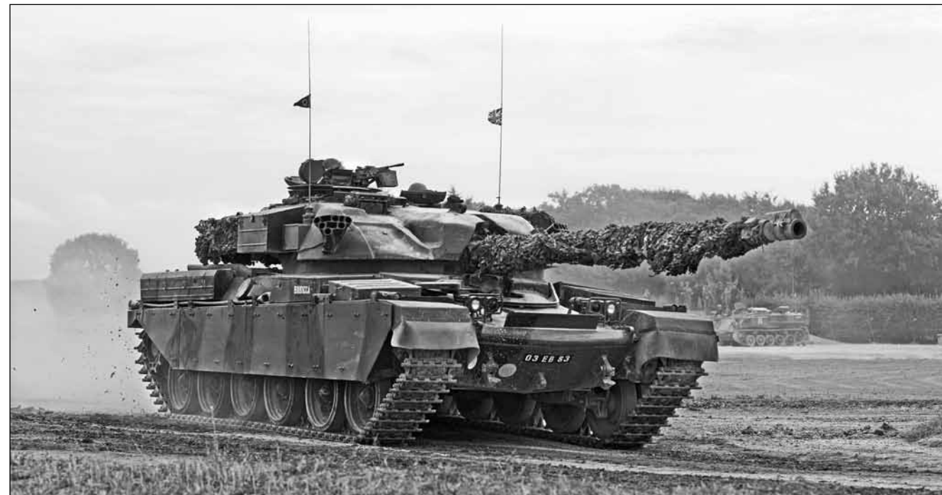
A Mk.11 Chieftain fitted with a Mk.13A L60 Sundance engine. This engine was rated at 720 bhp @ 2250 rpm. There was a more powerful version available for overseas sales but differences in engine specification ie. a three lobed Roots blower instead of two lobed would have increased the British Army's spares holdings (Peter Trimming from Croydon, England)
