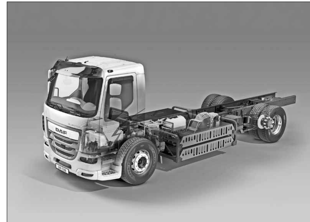
A 'Ghost View' of the DAF LF Electric
