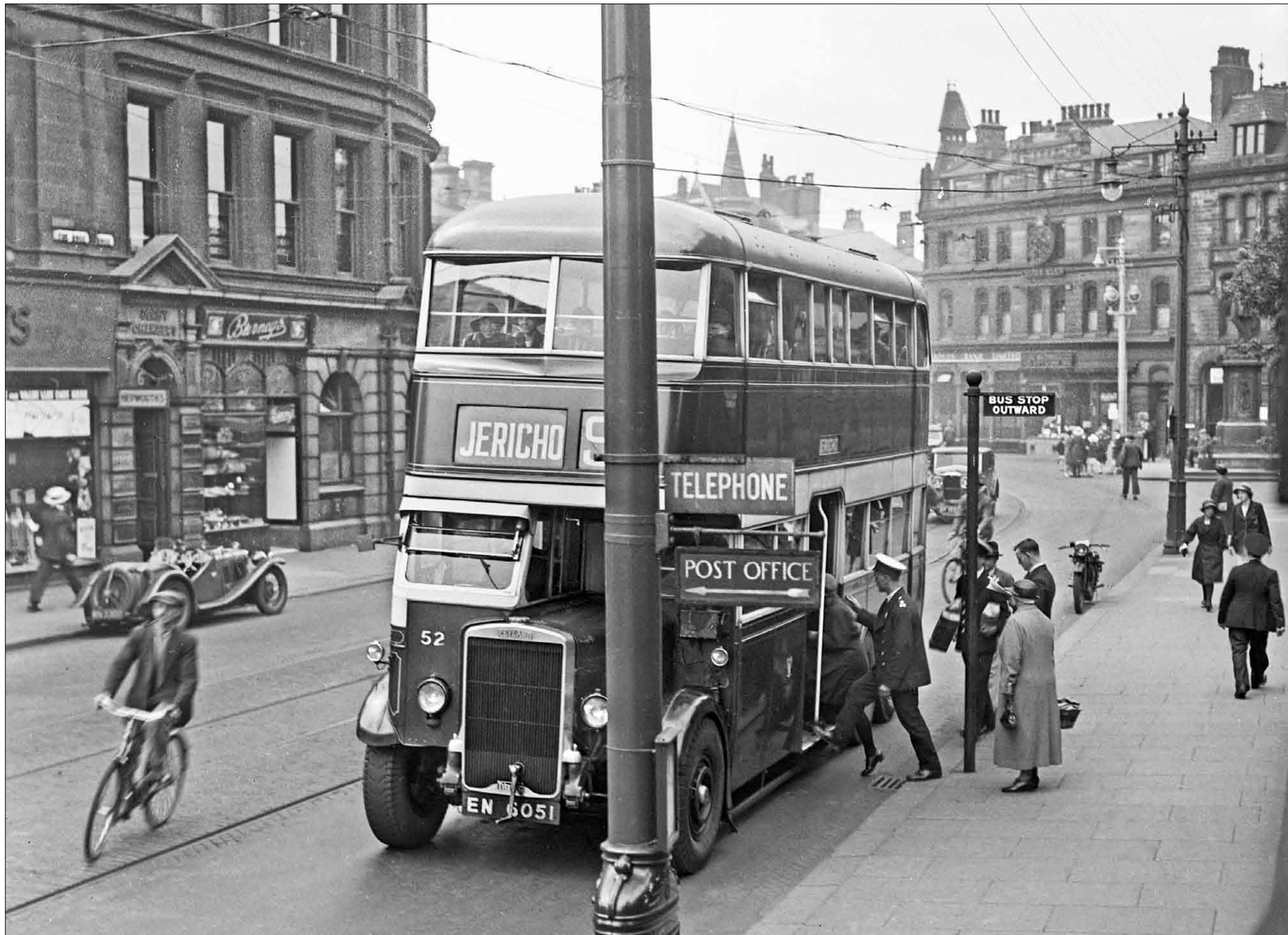
Oddly, the Leyland Titanic designations did not follow the sequence used for the Titans. Bury Corporation 52, EN 6051, was a model TT2, chassis 5156, with EEC coachwork – see also page 40
