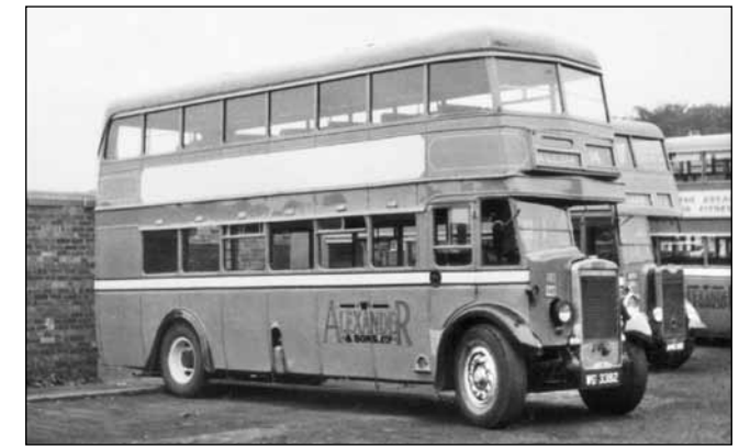
R48 after rebuilding and transfer from Perth to Alloa Depot. Again, the wide pillar behind the driver's door can be seen and the application of sliding vents.
