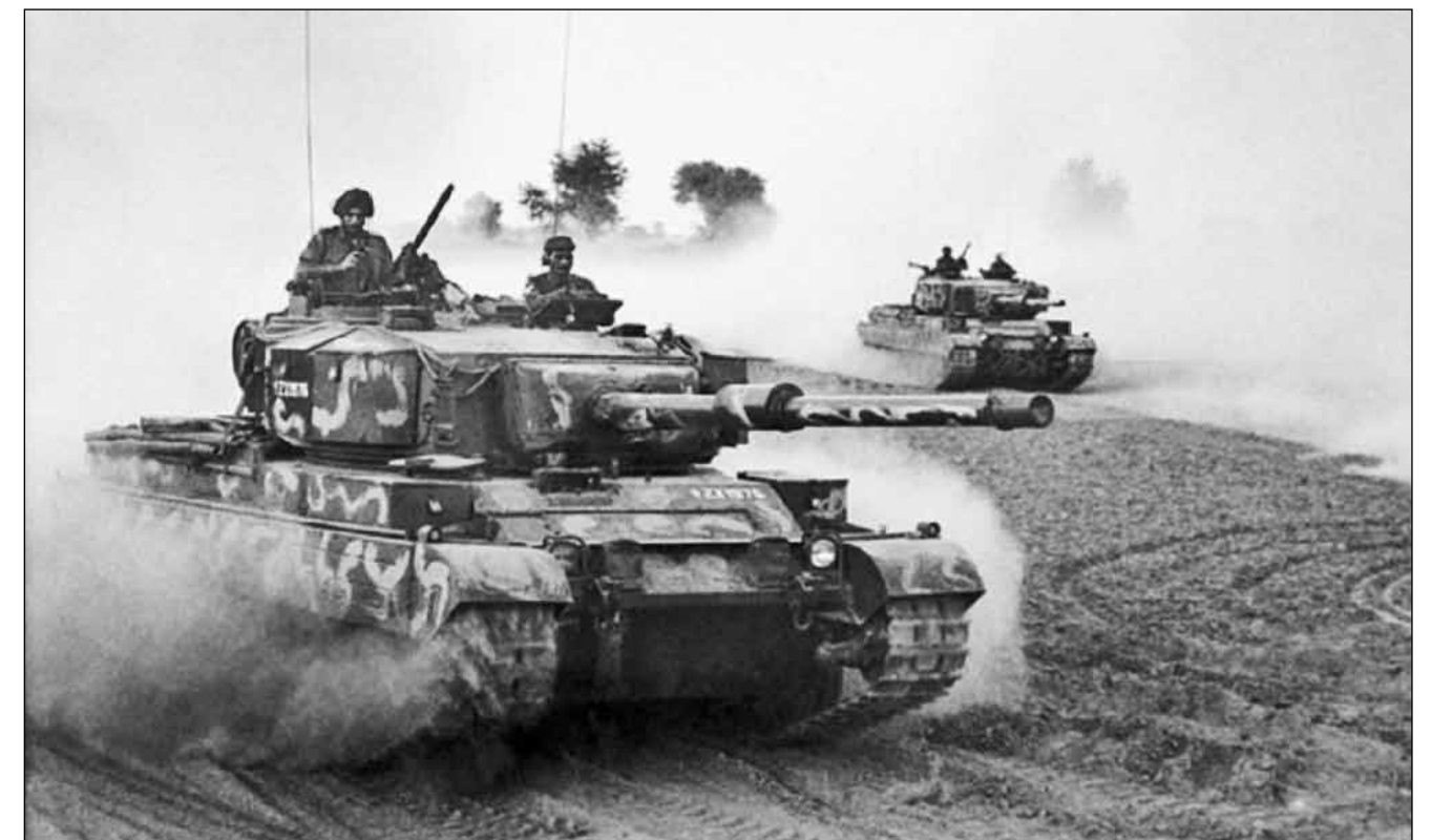
A Vijayanta tank in service with the Indian Army. This photograph shows the extremely dusty conditions that the vehicle was expected to operate in and clearly demonstrates the need for good air filtration to prevent damage to the engine (Image reproduced with the permission of 21st Century Asian Arms Race)
