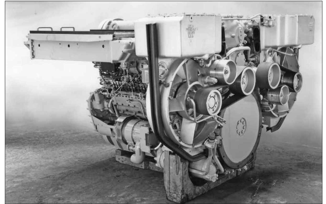
View of a post Sundance exercise engine for comparison. The drive belts are now ribbed rather than toothed and only the left-hand fan assembly contains a sprag clutch, the right hand fan now being a solid drive.
