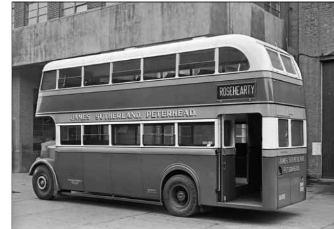
Manually operated doors were offered from 1949; an option taken up by customers such as Sutherland of Peterhead (BCVMT L032267)
