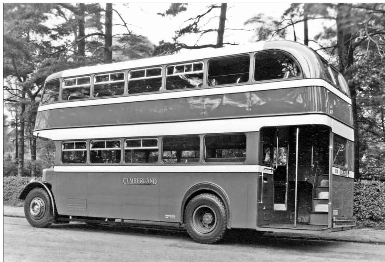
Cumberland 305 (KRM 254) was one of the few PD2s fitted with rear bumpers. These had been a feature in some fleets but the practice had largely died out by the date this bus was delivered. In later life they were removed.
