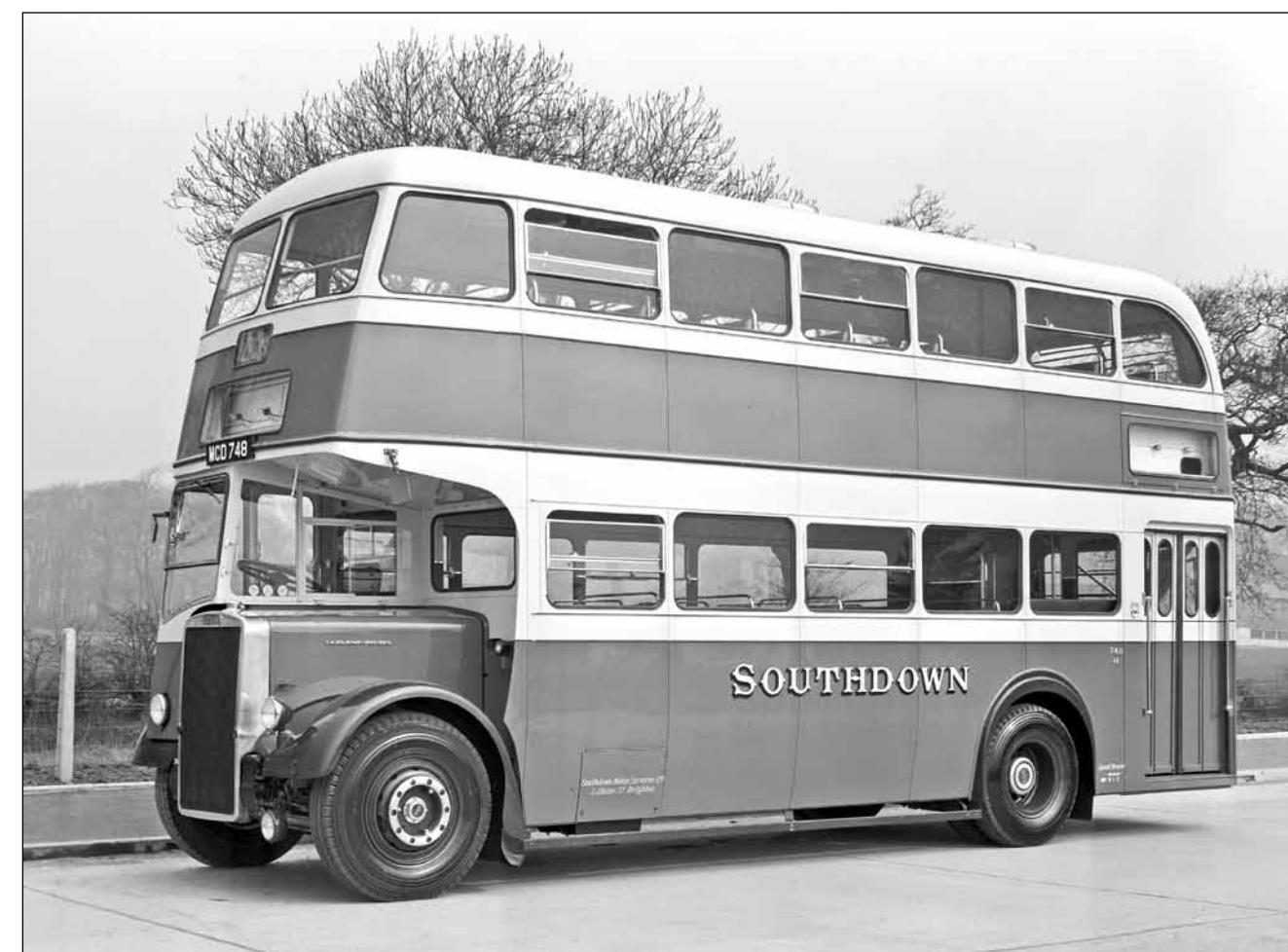
Southdown MCD 748 displays the half-drop windows option available on the 'final design' body and also the four part electrically powered doors. Leyland at its best – RTs? – not a patch on these magnificent buses – Ed! (BCVMT L046293)
