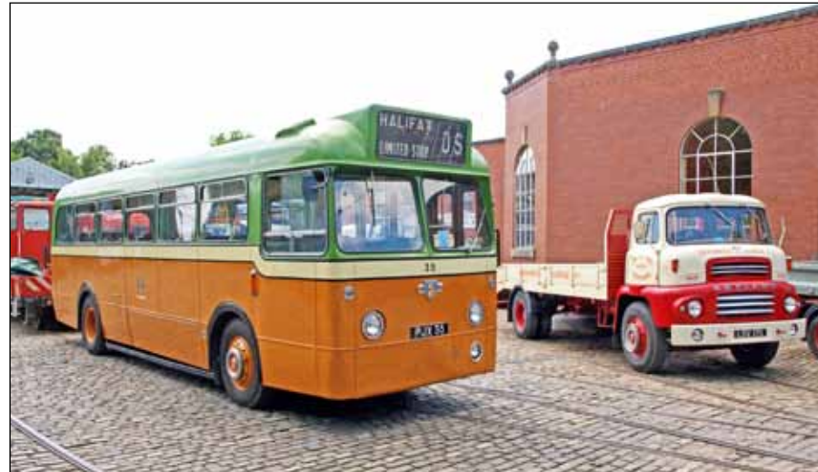
The rounded lines of the short door LAD cab fitted to the 1960 Comet show the contrast in construction technique when compared with the simpler design of the Weymann bus body of the 1961 Leopard L1, which was new to Halifax Corporation. (Gary Dwyer)
