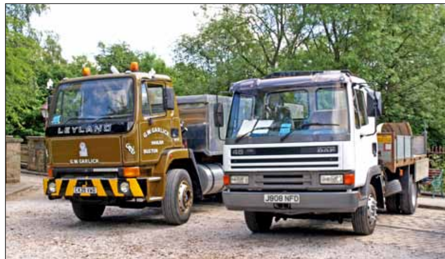
A pair of tippers contrast the simple lines of the earlier version of the C40 cab fitted to the 1985 Constructor 24.21 against the restyled grille fitted to the 45.130 produced in the Leyland DAF era, although the common parentage is clear. (Gary Dwyer)
