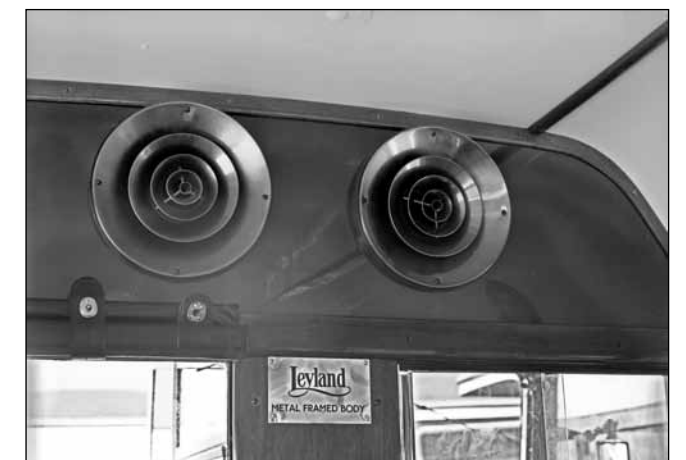
The lower deck front bulkhead of the Leyland body had two distinctive anodised aluminium circular ventilators and a brass badge showing its pedigree (BCVMT L032263)
