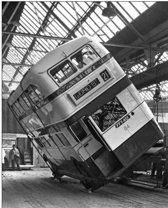
Below - Southport FFY 401 carried the original 8ft wide body. Note the famous Leyland 'S-shaped' drip moulding over the emergency exit, to reduce water falling over the platform area (BCVMT L033799)
