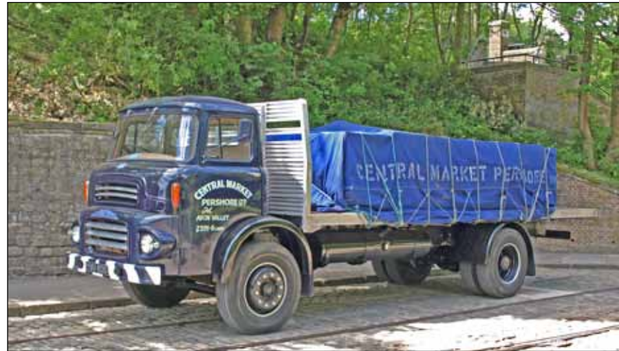
The long door version of the LAD cab is fitted to this Albion Clydesdale chassis with platform body and dummy load. Manufactured in 1969, it entered service with registration YWU 613G and is powered by a Leyland O.401 engine. (Gary Dwyer)
