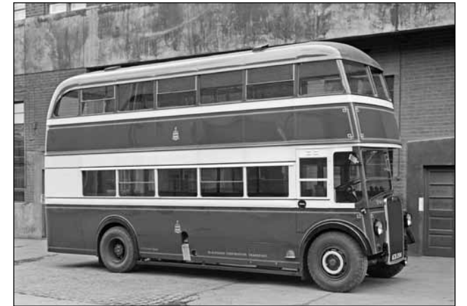
Blackburn Corporation ACB 206 carried one of the first post-war bodies to be constructed. It was among a batch of 50 sub-contracted to Alexander as the Leyland bodyshop was not available. Interestingly no front destination indicator was fitted but the vehicle was fully lined-out! (BCVMT L030530)
