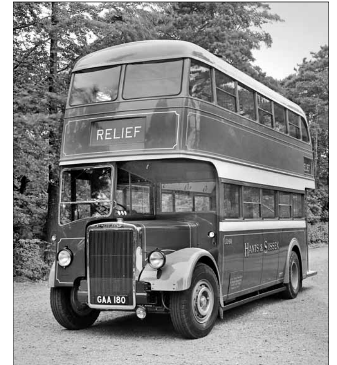
Hants & Sussex PD1, GAA 180, illustrates the 'simpler version of flush front upper deck windows' introduced to save construction costs (BCVMT L033247)
