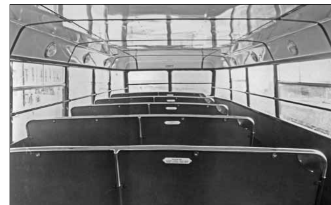
The updated body, introduced in 1950, had a double-skinned front dome which superseded the wooden inserts. This is shown to good effect on Ribble 1307 (BCVMT L041597)
