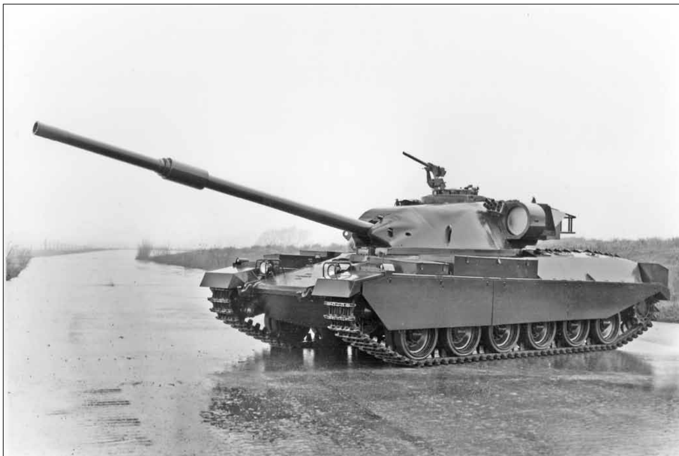
Left hand view of a prototype FV 4201. The lettering on the sloped front of the hull although difficult to discern appears to read "FHL FV340243 LML". All fighting vehicle components carried FV part numbers so it could be the part number of the hull or casting. The turret design is different from the design seen on the Mark 1 Chieftain and the gun is possibly a mock up. The large circular object attached to the turret was called a light projector (searchlight).
