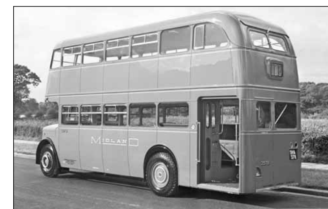
BMMO classified their vehicles as LD8. These PD2/12s, apart from their 'tin front', carried a slightly modified final version of the body, with smaller emergency exit windows, as seen here on SHA 378
