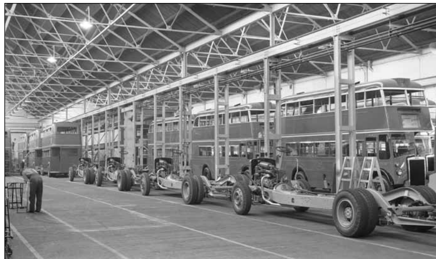
London Transport STD class vehicles nearing completion. These had PD1 chassis (BCVMT L031040)
