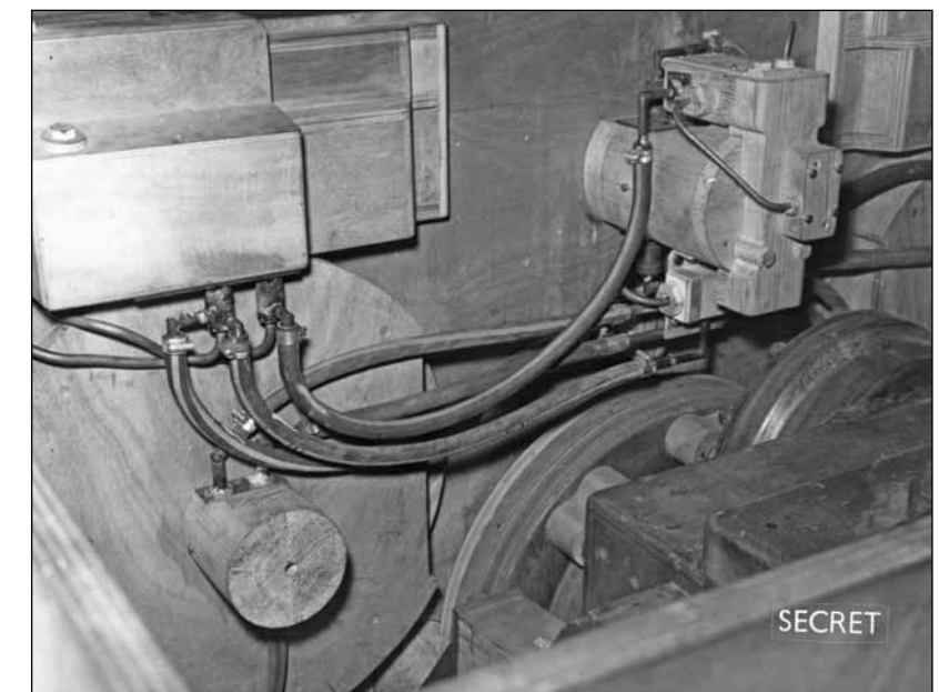
This is a photo of a wooden mock-up of part of the L60 engine. It is dated 17.09.59 and carries the ID F.V.D.E. 43352 2. It was common practice for components to be initially made in wood so that design engineers could check clearances, pipe runs and any assembly issues and this practice continued at Leyland well into the 1980s (there was a joiners shop at the Leyland Technical Centre). Although the details on the photo don't identify the location on the engine it is possibly part of the hydraulic system.
