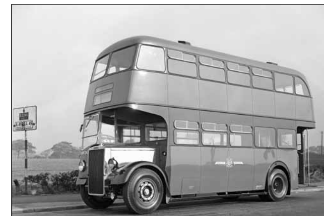
A front nearside view of the Farington body. This example was a PD2/1 for Leeds (BCVMT L039246)
