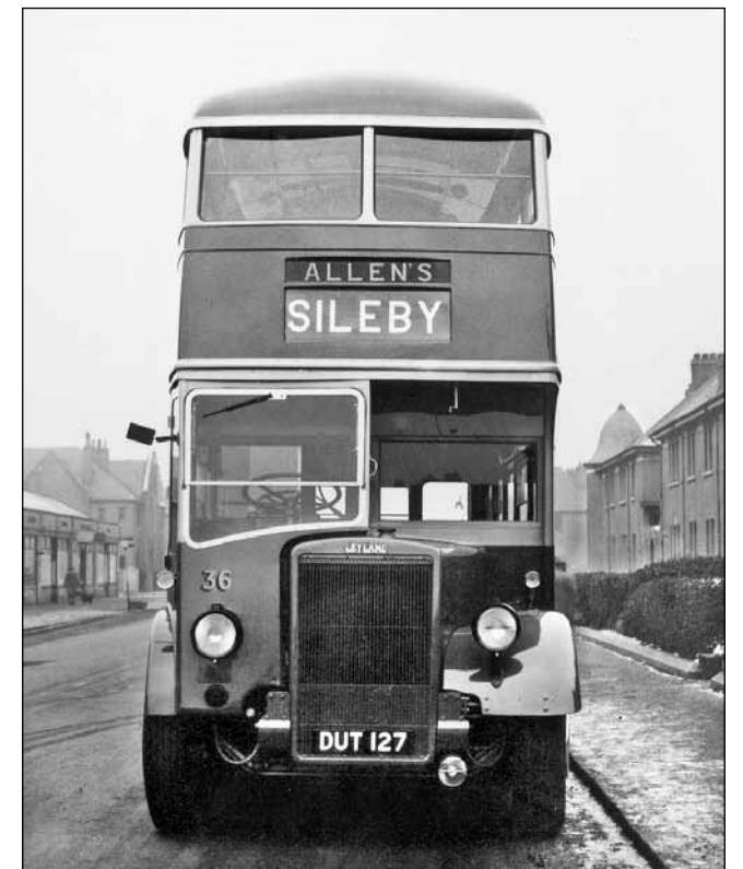
The interior lighting in Alexander built bodies was fitted in the roof rather than the cove panels used in all Leyland bodies. These can be seen in this view of DUT 127 of Allen, Mounsorrel. Compare with view of Rees & Williams' PD1, below (Allan Condie collection)
