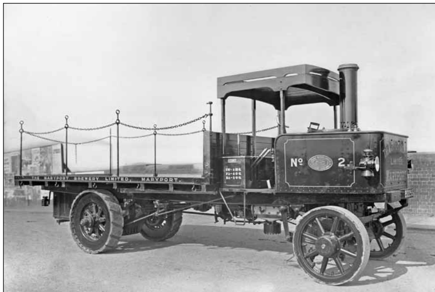
Leyland introduced the Class K shaft-driven steam wagon in 1909 with under-type engine connected by a shaft to a live bevel driven back axle. There was the KX 4ton and KW 6ton, but they were not a success with only 9 built – see Journal No.5 (BCVMT LB0665)
