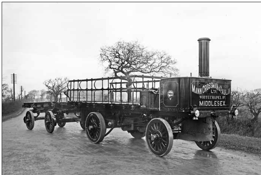
Mann, Crossman & Paulin, Whitechapel, Middx, were good customers of the LSMCo. This is their first Class B wagon, supplied in December 1902 (before registration numbers, later A 966). The weight at 2.19.0 was 'kept under 3 tons' by the signwriter! (BCVMT LB0123)
