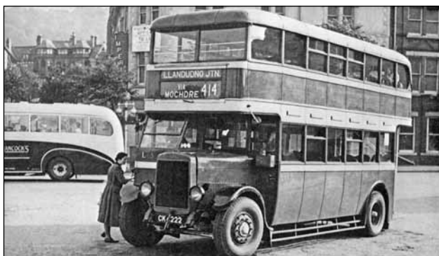
Leyland TD1, CK 4222, with ex-Cardiff NCME body from a TD2 (Mike Sutcliffe collection)
