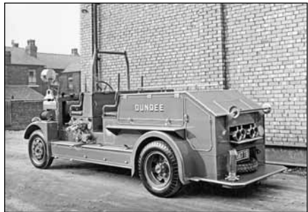
A nice near-side view of the FK7, YJ 4036. Note the side mounted pump and the stowage arrangements for the suction hose, the strainer next to the spare wheel and on the rear body the trunnion which together with the U gantry for the escape head allowed a wheeled escape to be carried. The appliance is carrying Lancashire CC Trade Plates (BCVMT L018379/80)
