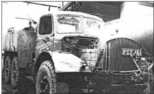
The Mack conversion to an O.680 engine
