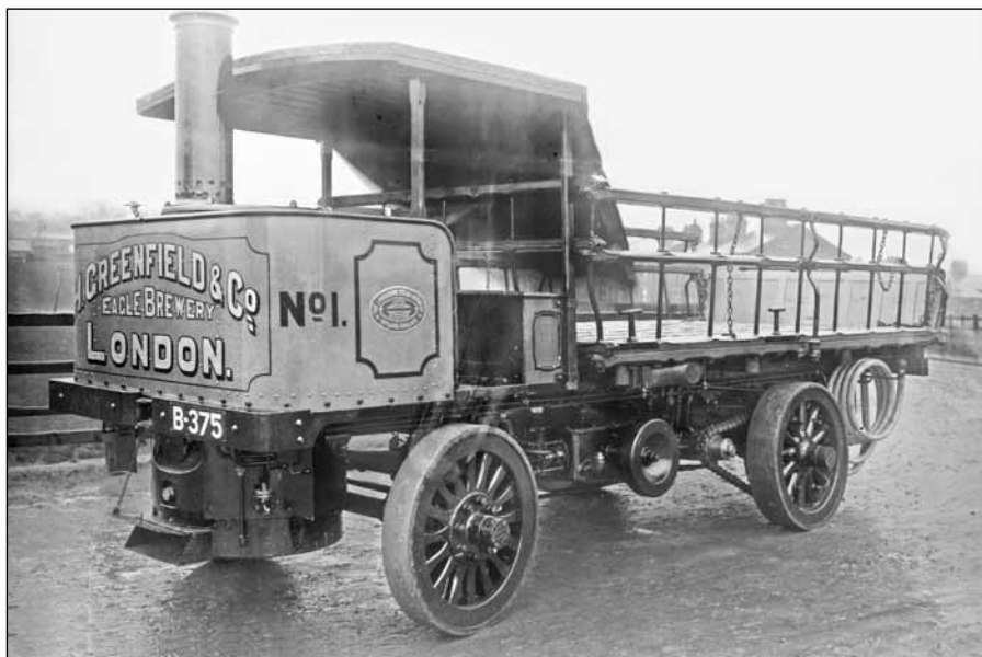
B 375 was registered in March 1904 to H Greenfield & Co (Eagle Brewery), London. It was another Class B wagon and had a flywheel on the nearside of its under-type engine. It had composite hind wheels but timber front wheels and steel tyres. (BCVMT LB0213)
