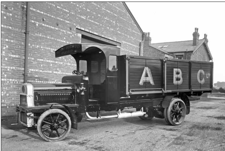
The Aylesbury Brewery Co went in for the heavier model, the X2.40.W, with the Class W axle which had the bent 'I' beam under the 'axle gearbox' and bevel drive for carrying weights of 5-6tons. The body was a high-sided tipper (BCVMT LB0957)
