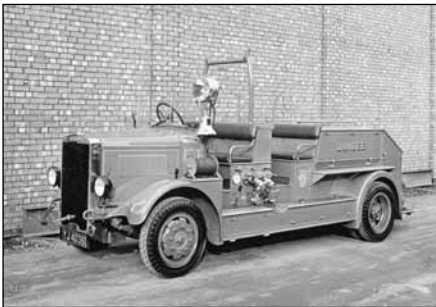
A nice near-side view of the FK7, YJ 4036. Note the side mounted pump and the stowage arrangements for the suction hose, the strainer next to the spare wheel and on the rear body the trunnion which together with the U gantry for the escape head allowed a wheeled escape to be carried. The appliance is carrying Lancashire CC Trade Plates (BCVMT L018379/80)
