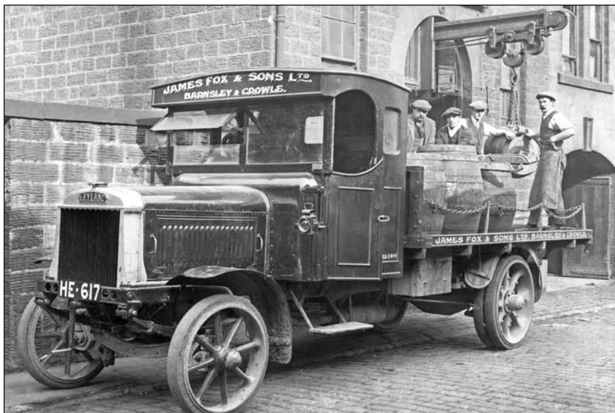
The model K was basically a model G but with the lower radiator and longer bonnet (18 louvres rather than 16) which enabled the larger 40/50hp X4.40hp engine to be fitted as an extra if required. HE 617 belonged to J Fox & Sons, Barnsley & Crowle (BCVMT L000380)
