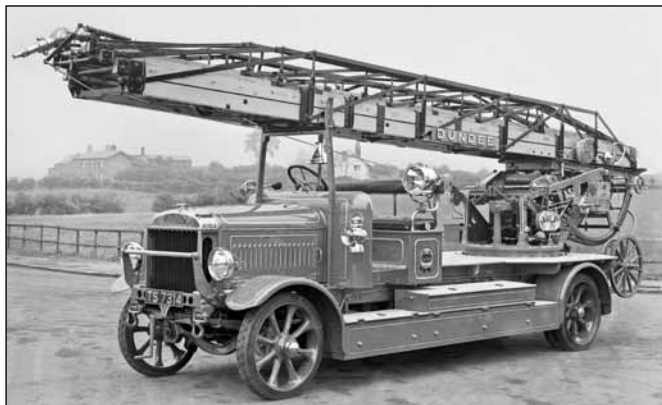
The Leyland F.E.2 Special with Carl Metz 85ft turntable ladder (BCVMT L005092)
