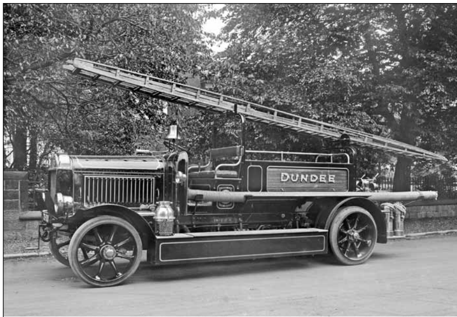
Dundee's first Leyland Fire Engine in 1915. It was unusual in that it had the X4 type radiator and the heavier X4 chassis frame (BCVMT LB1681)
