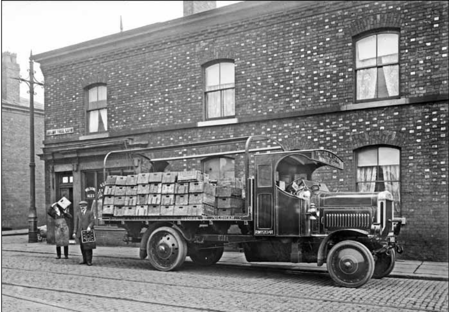
B 8592, a very early 1919 Leyland G of Taylor & Lees, Oldham, being unloaded in Hulme Hall Lane, Manchester. Note the Manchester licence 'P.Mcr.2134/1' painted on the cab and the enormous gearbox under-tray to catch the drips of oil (BCVMT L000018)
