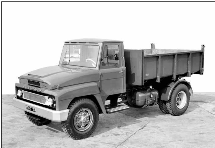
This 1966 prototype bonneted Super Comet Truck was developed specifically for Iran with a new design of cab to replace the split screen cab already produced in Iran (BCVMT L090549)
