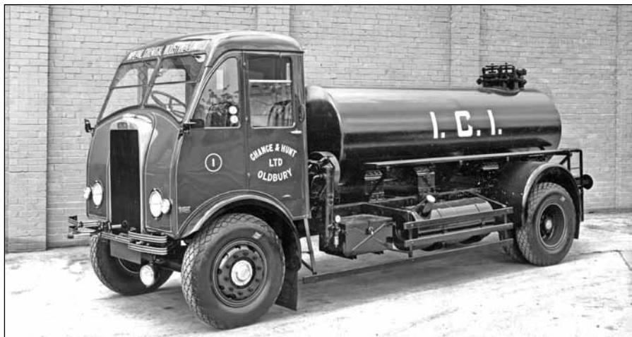
The same ICI Leyland Beaver TSC8 tanker as seen on the previous page in the Running Shop. Note the streamlined cab, possibly built specially for ICI. It is not unlike the streamlining of the ICI six-wheeled Cub fire engine / foam sprayer, shown in a scrapyard on the opposite page (BCVMT L021835)
